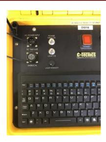
The above Picture shows the labelling of the female ends of the C-Technics C-Vision Box with the Upper Fitting Being the AC Power and the Lower fitting being the Camera Umbilical Fitting. You will notice the internal seating on the female ends which should be checked and matched up appropriately. The AC Power Input lead is Yellow. This should be visually inspected prior to use and placed in placed in the Peli case when not in use.
