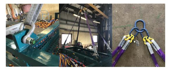
The above pictures show how the various parts of the lifting arrangement should look. Once these checks have been completed, then the Frame should be prepared for lifting. It is important that the rigging is not twisted and is only lifted from the designated central Masterlink as shown in the picture on the right.
