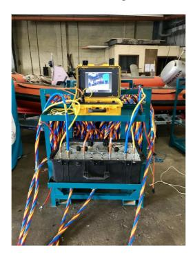
The above picture shows the configuration of the Diving Panel and hoses as they are fitted while sat on the Panel shelf on the frame. Ideally the Panel and C-Vision Box can be used on the frame in good conditions, but where it is practicable then should be used in a Wheelhouse or Shed to protect all equipment from the elements. Prior to installing any equipment on the vessel, it is important to get permission from the contractor to install before beginning any wheelhouse instillations.
