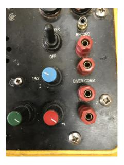
The Red Communication Connection should be connected to the Comms Box. Care should be taken That Diver 1 is plugged to Diver 1 input and likewise for Diver 2. These are labelled and a Comms check on both Divers will be carried out to function check these prior to any Diving operations commencing. Above is a photo of the Comms Boxes highlighting the Diver 1 and 2 Comms Cable inputs for both the SMP and Chamber Oceanic Boxes.
